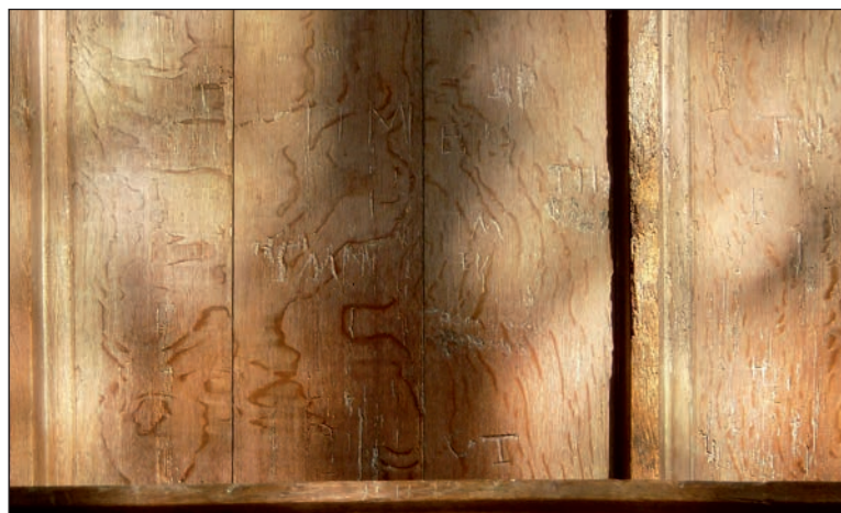
Fig. 12: An example of medullary rays from quartered oak. Medullary rays extend vertically through the tree across and perpendicular to the growth rings and allow the radial transmission of sap. When wood is quarter sawn (cut with the rings perpendicular to the face of the board) the medullary rays can produce beautiful patterns. Panels would often be selected merely because of the visual quality of their medullary rays. This would suggest that such panels were never intended to be painted.
