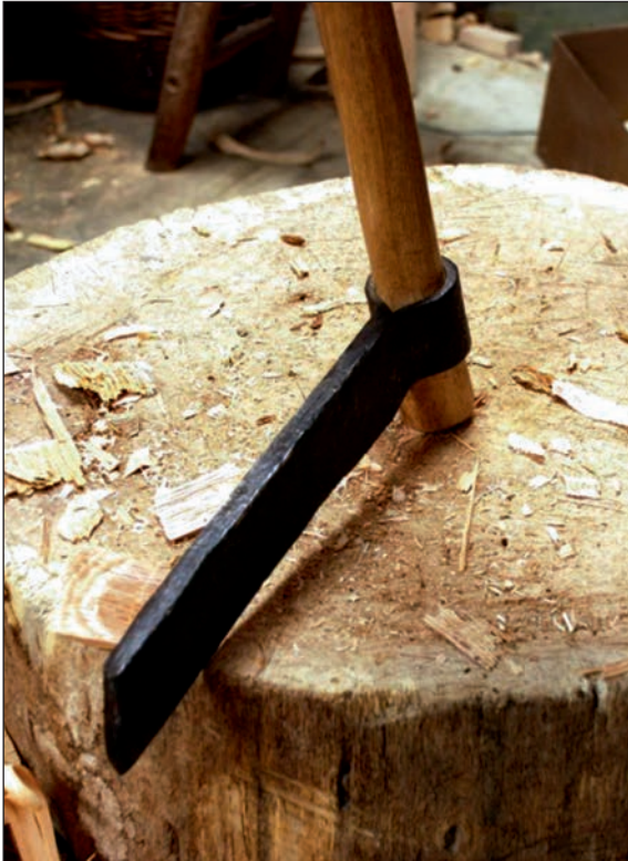
Fig. 10a (top left): Cleaving quartered oak with a froe to produce quartered shingles and, with larger sections of timber, wainscot panels. Notice how the wainscot is wedge-shaped at this stage in the process – thicker at one side than the other. Because the oak is quartered (split across the rings) the expansion and contraction with changes in humidity are reduced and it will be much less prone to warp as it dries out.
